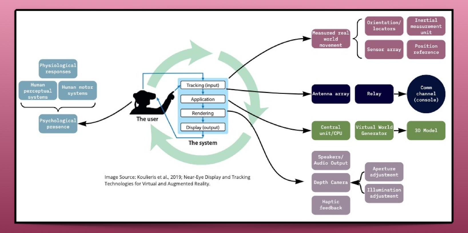
The above diagram deblackboxes the input-output cycle as well as the soft and hardware elements that make these four main processes possible. All together, they constitute VR's technical structure.
